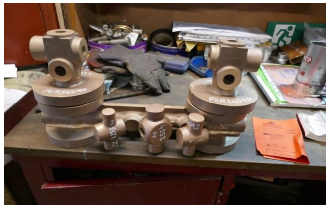
We are way ahead of the game with these gauge frame castings which are currently away for machining.
