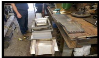
Water injector trays, which fit inside the boiler, ready to be fitted.
