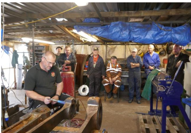
Scott Parker, during a quiet few minutes, melts the white metal thrust faces off the rods - with the Sunday team apparently being caught at a slack moment . . . again.
