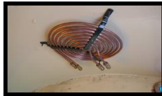
The condenser coil fitted to the cab roof which is part of the steam lubrication system.
