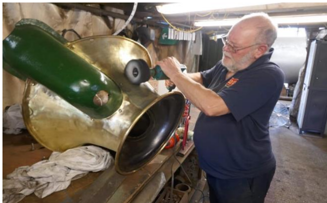
Pete Hubbard in action with his buffing wheel, giving the bonnet a final finish.
