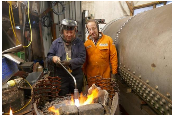
"Think that chestnut is done Martin!" Paul holding the torch on our mobile forge - heating lap seam rivets . . . we think?
