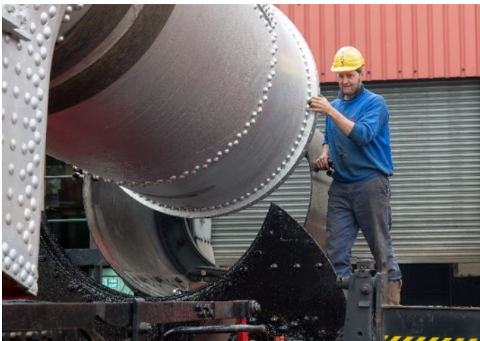
Henry guides the boiler barrel carefully into the smokebox. With the boiler and smokebox once again reunited, we were able to drill locating holes for temporary bolts, and there was never any doubt . . . it fitted perfectly!
