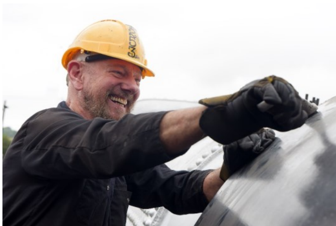
Henry guides the boiler barrel carefully into the smokebox. With the boiler and smokebox once again reunited, we were able to drill locating holes for temporary bolts, and there was never any doubt . . . it fitted perfectly!
