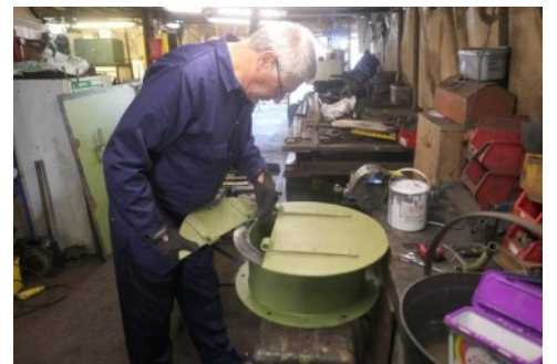
The new back panel with reclaimed brackets and steps riveted, sand boxes fitted and filler lid test fitted.
