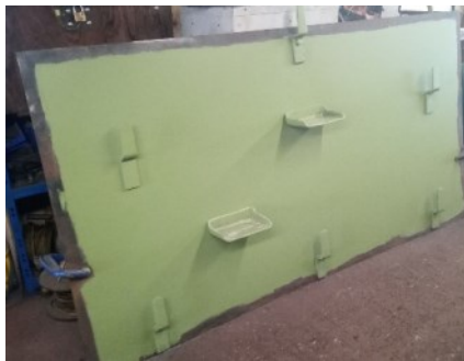
The new back panel with reclaimed brackets and steps riveted, sand boxes fitted and filler lid test fitted.
