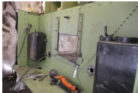
The new back panel with reclaimed brackets and steps riveted, sand boxes fitted and filler lid test fitted.
