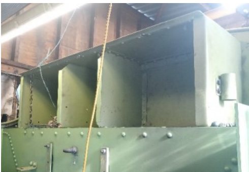
Tool boxes rivetted in place awaiting their doors.
